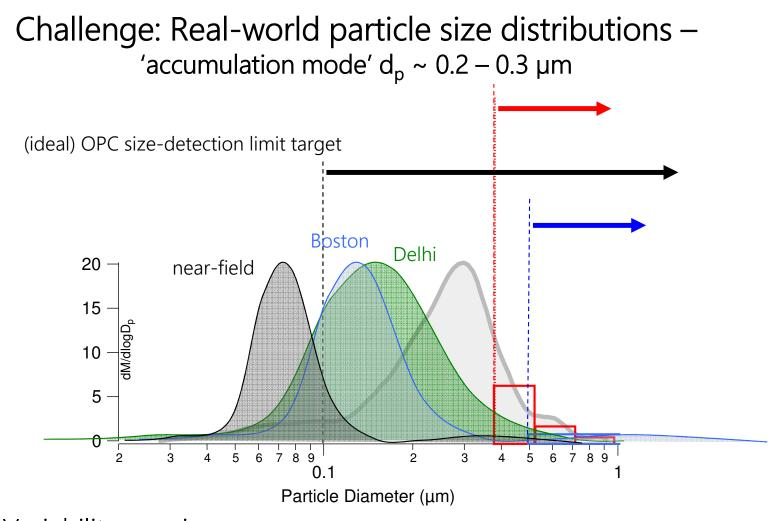
Variability in the SiZe distribution of ambient particulate matter changes the fraction of suspended PM detected by the low-cost OPC
