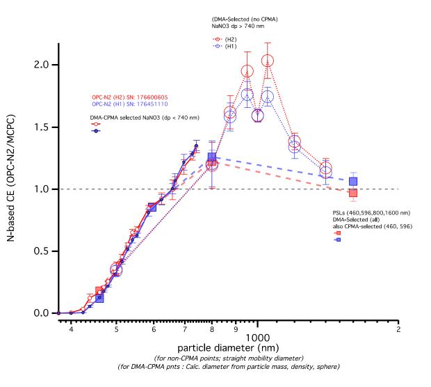
Number-based size detection efficiency of the two OPC-N2 units is  $LOD_{50} \sim 550$  nm
