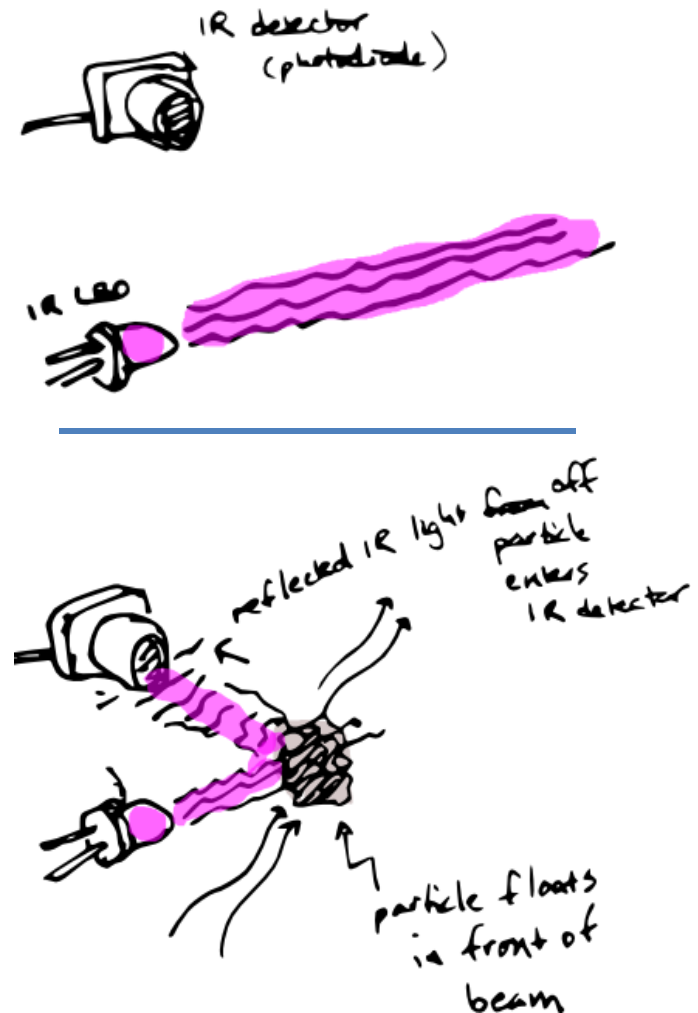
Above: Optical (light scattering) sensor (Dustino) Right: How it works
